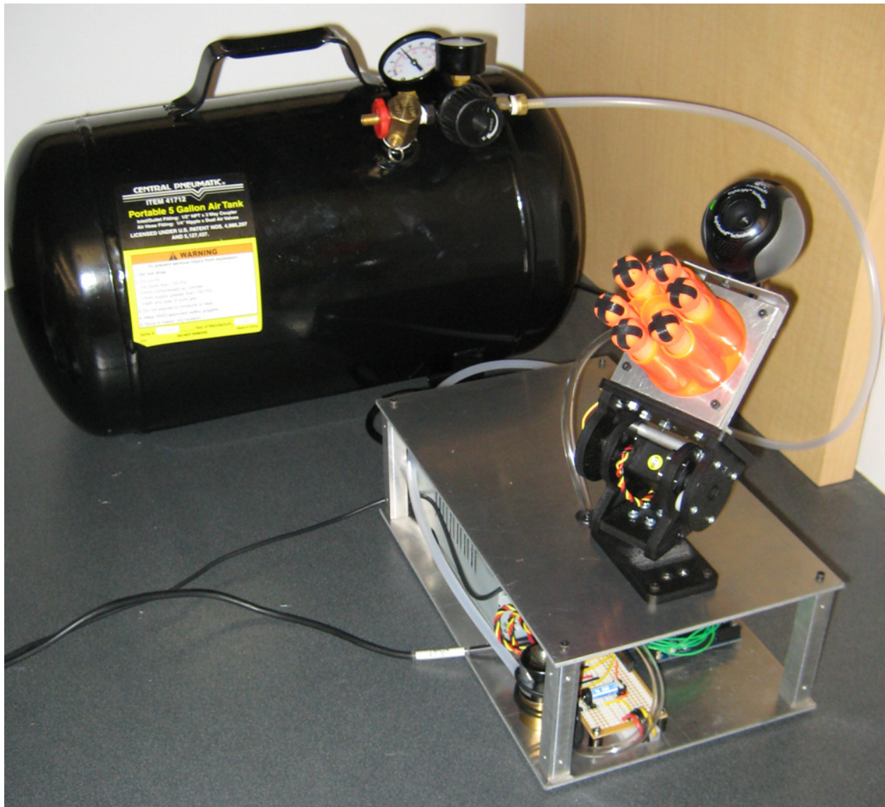
Figure 1: Completed Remote Controlled Turret
